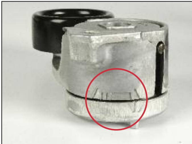
Look for the Tensioner Belt Wear Indicator found on many Automatic Belt Tensioners
